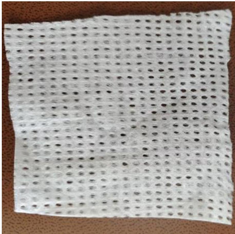
图 1. 克重 60, 全棉 8 目网眼水刺非织造布 Figure 1. Cotton spunlace nonwoven fabric with a grammage of 60 g/m 2 and 8-mesh apertures
