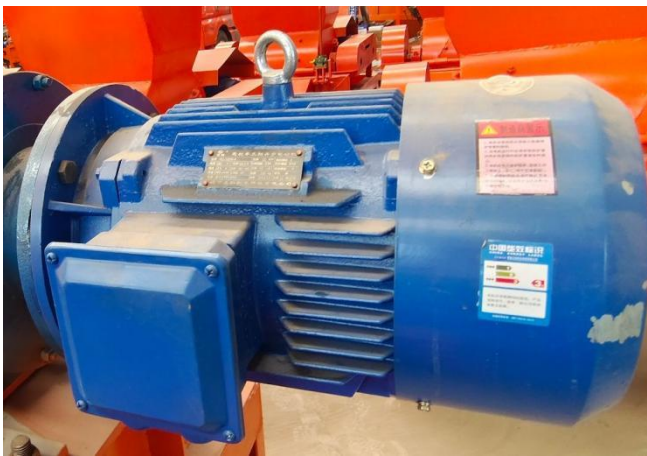
图2 YE3-160M-4 电动机 Figure 2. YE3-160M-4 Electric Motor
