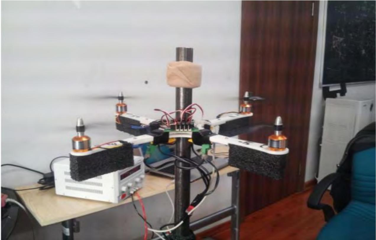
Figure 6. Dynamic test stand for the elaboration of control parameters for a quadcopter in Mongolia [6]
