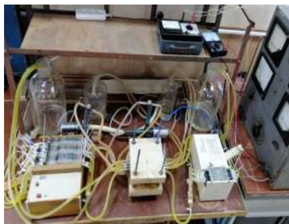
Figure 3 – General view of the electro-dialysis unit
